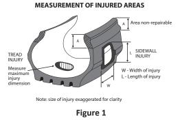
For both bias and radial ply tires, refer to the repair material manufacturer's repair unit selection chart for appropriate repairable injury size and repair unit selection.
