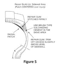
For bias ply tires, the repair unit should be installed so that the platform of the repair unit, where the reinforcement plies intersect, extends 25% past the extent of the injury.
