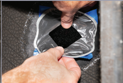
Place Repair Unit Over Cemented Area
