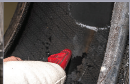
Vacuum Debris (without contacting buffed surface)
