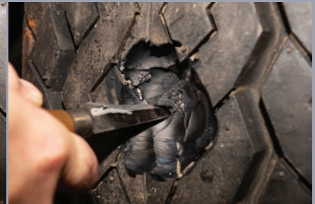
Use Knife to Remove Loose or Damaged Rubber
