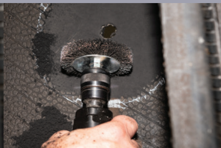
Remove Buffing Dust With a Fine Wire Brush
