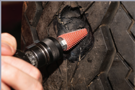
Use a Coarse-Grit Rasp to Remove Damaged Rubber
