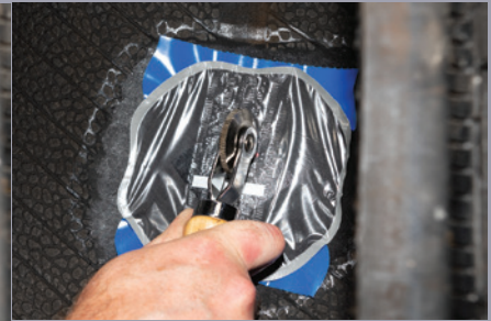
Stitch Repair Unit From the Center Out
