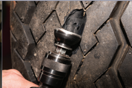
Skive to Remove Damaged Rubber and Cord Material
