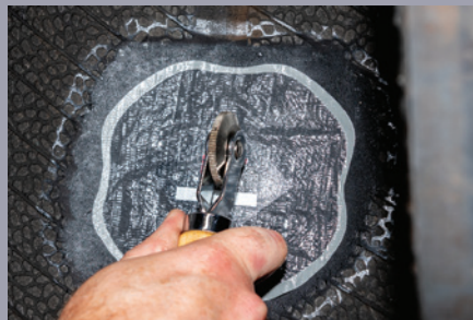
Remove Protective Film and Check for Proper Installation
