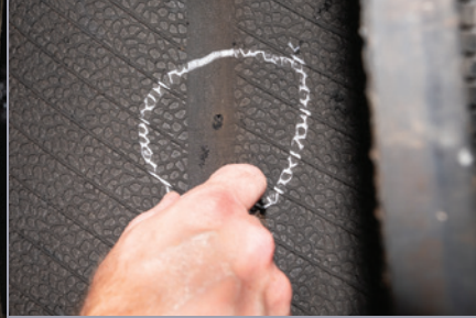
Mark Repair Area for Cleaning and Buffing - Inside Tire
