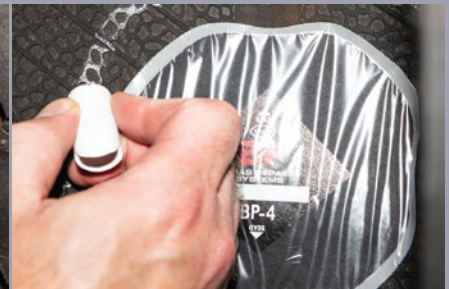
Measure the Injury and Trace Around Repair Unit
