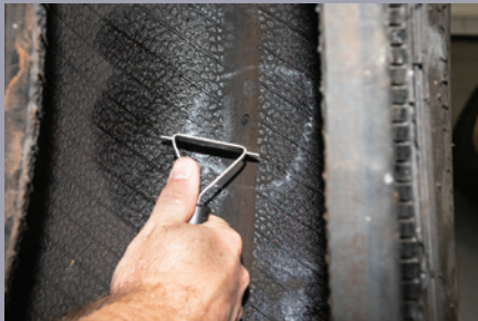
Scrape Repair Area Inside Tire
