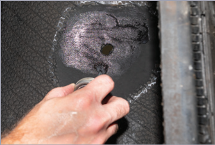
Apply Cement to Inner Liner and Skived Area
